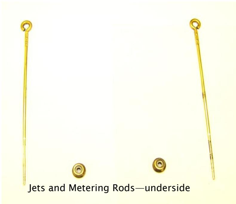
Jets and Metering Rods—underside
